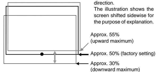
\* The projection position can only shift in an up-and-down direction.
